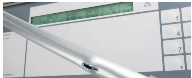
Result of a burst pressure test with the universal pipe RAUTITAN Flex
